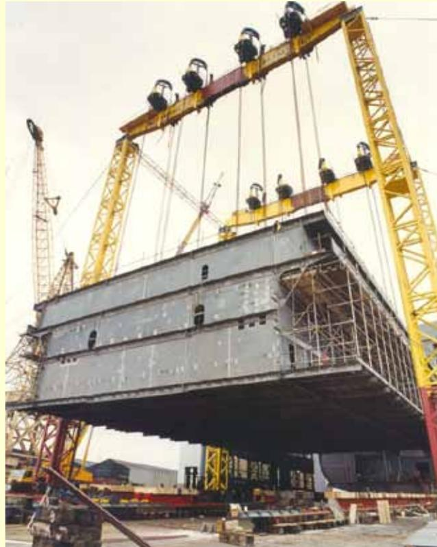
Note skid beams prepared for skidding of lower hull
