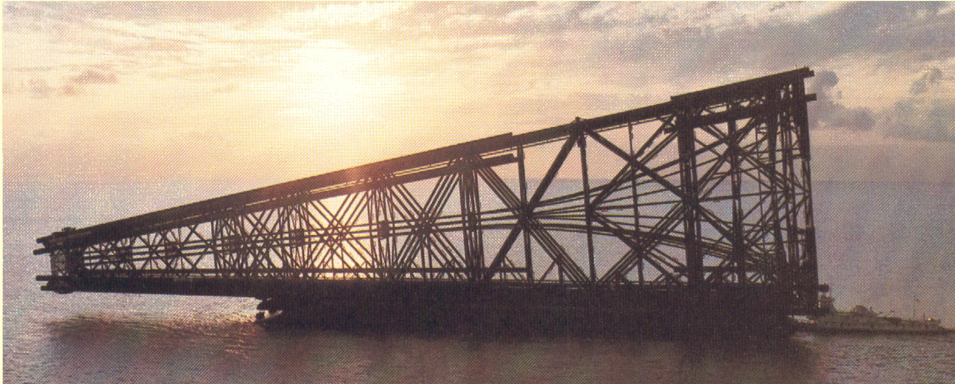
Note the need to check for tow fatigue resulting from large stress ranges imposed on the connections for long and stormy voyage
