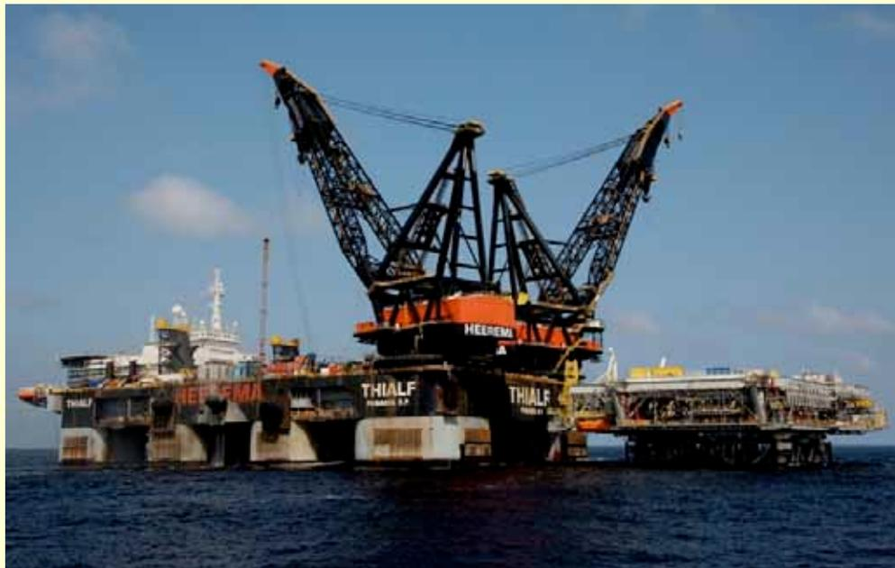
**Dual crane-4 lift point lift**
