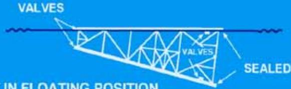
2 CRANE LIFTS JACKET AT TOP AND VALVES ARE OPENED
